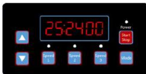
(Diagram 6.16, schema 2 hastighet, standard 2400rpm)
