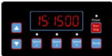
(Diagram 6.12, schema 1 Hastighet, standard 1500rpm)
